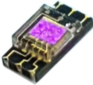
HLALS026AC-K1 is a light to digital converter which combines photodiodes, current amplifiers, analog circuit and digital signal processor.
